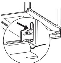
Open the door fully and hold the two door hinges.
