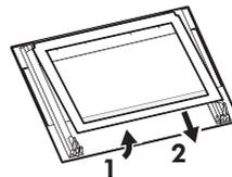
First lift carefully and then remove the glass panel.
