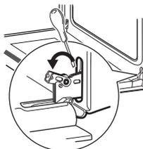
Lift and turn the levers on the two hinges with a screwdriver.
