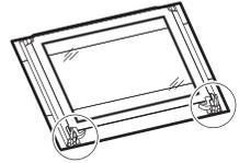
Put the door on a soft cloth on a stable surface.
